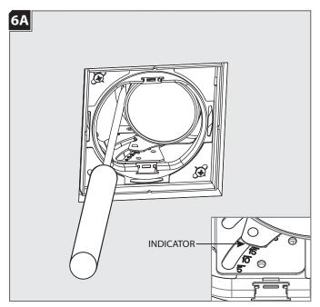
To tilt the module, use a long screwdriver to gently push the module to the desired angle.
