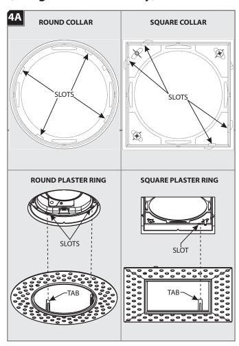
Align the plaster ring tabs with the slots in the housing. Push the tabs up through the slots and bring the plaster ring flush to the ceiling. All four alignment tabs must be on the inside of the collar and through the slots. The plaster ring should be centered to the housing aperture.
