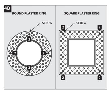
Secure the plaster ring in place with the four provided self-drilling screws appropriate for your drywall thickness. The four mounting holes on the ring are smaller than the plaster holes. Make sure that the screws penetrate through the fixture housing.
