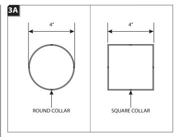
Mark an appropriate sized diameter circle or square on drywall. Cut out the marked section. **Note:** The drywall may be cut by running a 1/8" RotoZip around the outside of the collar.
