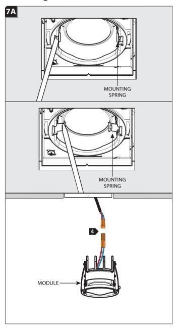
**Note:** The module must be removed in order to access the junction box or replace the optic.
