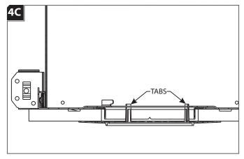
3 The top portion of the alignment tabs on the plaster ring should be broken off to avoid interference with the light module. Bend the tabs back and forth inside the housing to break the tabs.
